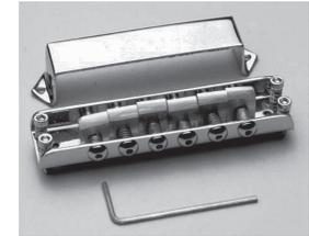
To raise the height of the strings from the surface of the neck, raise the bridge by turning each of the four adjusting screws clockwise using the adjusting key supplied with the instrument. Lower the playing action by turning the adjusting screws counterclockwise.
