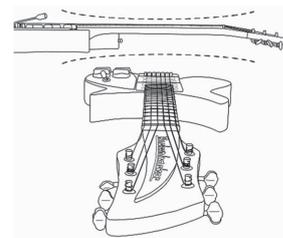
Should adjustment be necessary, take the strings out of the nut grooves to allow room to remove the nameplate from the head of the instrument. After replacing strings to the grooves of the nut, retune the instrument to assure normal tension on the neck.
