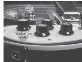
Modern 4003 Series basses now allow this capacitor to be easily added or removed from the circuit. With a simple upwards pull of the treble tone control, the Vintage
